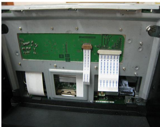
STEP 8: Slot supplied Cable in to the disassemble place.
